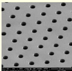
**Figure 1. SEM image of CellSieve™ microfilters with 7- $\mu$ m diameter pores in a uniform array.**
