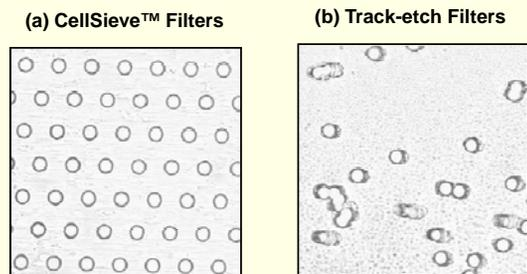
**Figure 1.** (a) CellSieve™ microfilter fabricated by lithography method with regularly distributed pores, and (b) track-etch filter with random pore distributed pores.
